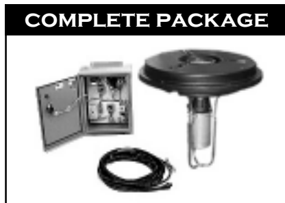
U.S. Package: Unit, NEMA 3R Power Panel (with timer, GFCI (except 460V), breaker, surge arrester, HOA switch and thermal overload protection), 50 ft. of SOOW cable. Int'l Package: Unit and 15m of cable (no cable on CE).
